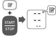
• All readings will be deleted. You cannot partially delete the readings stored in the memory.
